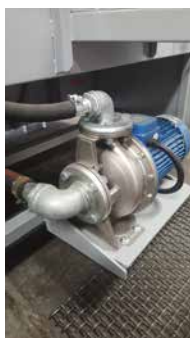
Easy access pump for rapid service removal
