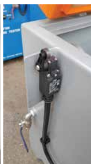
Safety lid switch cuts out during cycle
